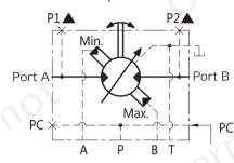
CS: Control pressure from port A or port B with shuttle valve
